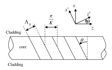
Fig. 1. Configuration of tilted fiber grating.
