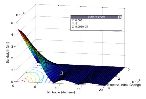
Fig. 3. Bandwidth of tilted gratings versus tilt angle and effective index change when  $r_{\rm max} = 0.95$ .
