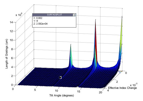
Fig. 4 Length of tilted gratings versus tilt angle and effective index
