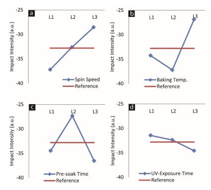
Fig. 2 Effect of different levels of factor (a) spin speed, (b) baking temperature, (c) pre-soak time in developer, and (d) UV exposure time.
