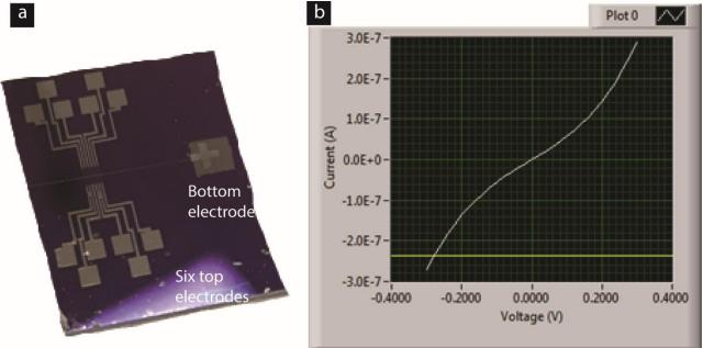
**Figure. 3** (a) Tunnel junctions where bottom electrode is deposited in the optimized photoresist protocol to remove notches along the edges. (b)Current-voltage study showing the realization of tunneling behavior between top and bottom metal electrodes.
