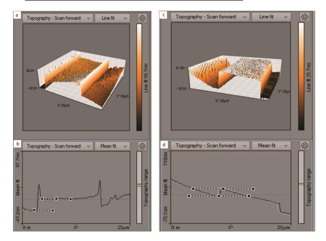
**Figure 1** AFM images notches before and after the optimization of photolithography process. (a) 3D image and (b) cross section view of patterned thin film with notches along the side edges. Side edges are result of improper photolithography conditions (c) 3D and (cross sectional view of patterned thin film with no sharp notches along the side edges. Notch free edges are result of optimized photolithography parameters.
