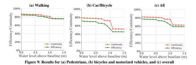
Moreover, floods that exceed 1.0 m from the baseline impose major decreases in the metrics for the network, with 55% of car routes being blocked and the efficiency of paths falling to 50%, which means the routes during the events are twice as long on average. For pedestrians, on the other hand, there are no large dips in the curves. This is another evidence that motorized vehicles are more vulnerable to blockages, particularly in arterial roads, which tend to create bottlenecks in the system.
