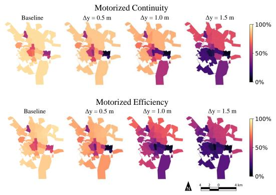
Figure 7: Motorized vehicle metrics. Darker shades indicate that a larger proportion of paths from/to the traffic zone are no longer possible after the flood.
