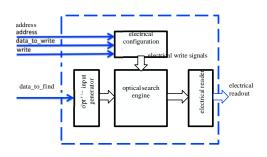
Fig. 2. Overview of the proposed optoelectronic CAM (OE-CAM).
