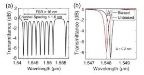
Fig. 9. (a) Transmitted optical power spectrum indicating the ring FSR of 16 nm and channel spacing of 1.6 nm. (b) Transmitted power versus wavelength for biased and unbiased ring modulator.
