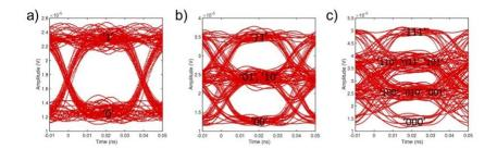
Fig. 10. Output eye diagrams of the EO-CAM for 25 Gbit/s modulation rates of silicon micro-ring modulators (for 1 (a),2 (b) and 3 (c) MRRs) with a Q-factor of 5000 and 1.6nm spacing between channels.
