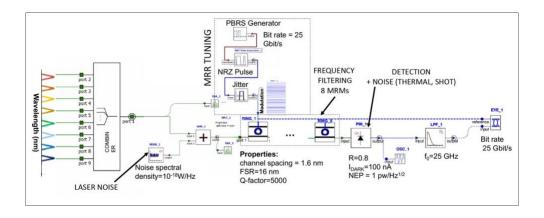
Fig. 8. Hierarchical schematic of a 8-bit OE-CAM. Writing and reading emulation.
