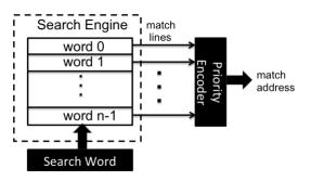
Fig. 1. Block diagram of a generic CAM.
