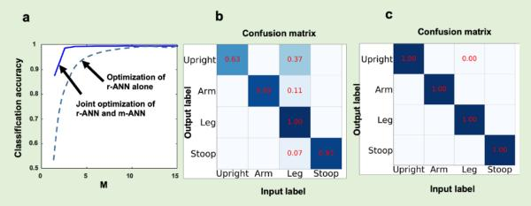
**Figure 4.** Selected experimental results of in-situ gesture recognition directly from a reduced number of measurements. (a) the dependence of the recognition accuracy on the number of coding patterns of the programmable metasurface. (b) The classification confusion matrix with the optimization of the r-ANN alone, where M=3. (c) The classification confusion matrix with the joint optimization of the r-ANN and m-ANN, where M=3.
