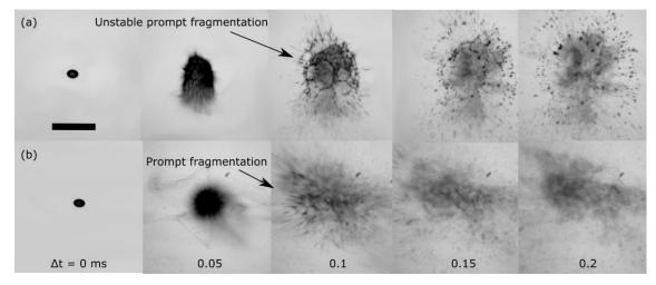
FIG. 18. (a) The transition from sheet formation to catastrophic breakup. (b) Catastrophic breakup. The scale bar indicates  $500 \,\mu$ m.
