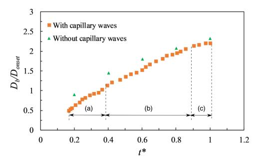
FIG. 9. The temporal evolution of bubble diameter  $(D_b)$  normalized with the droplet diameter at the onset of the nucleation  $(D_{onset})$  for droplets accompanied with and without the capillary waves. The bubble growth consists of three regimes indicating (a) bubble growth without stretching, (b) bubble growth with stretching, and (c) bubble growth with wave propagation.
