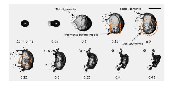
FIG. 16. Crown formation and the breakup of an emulsion droplet ( $D_{onset} \sim 0.3 \text{ mm}$ ) followed by capillary wave propagation on the sheet surface. The scale bar indicates 500 µm.
