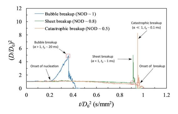
FIG. 6. Temporal evolution of droplet diameters resulting in bubble breakup, sheet breakup, and catastrophic breakup.  $D_0$  represents initial droplet diameter.
