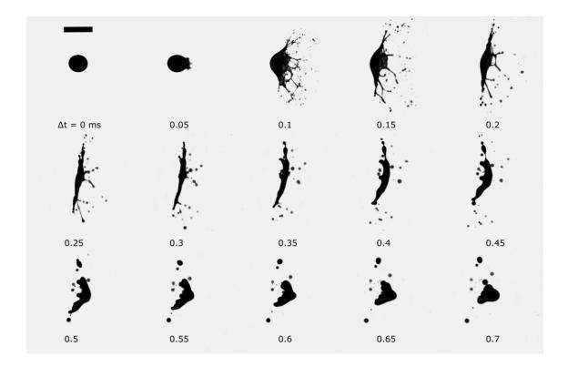
FIG. 17. Expansion of crown sheet and its reversal due to the breakup-induced reactionary thrust. The scale bar indicates  $500 \,\mu$ m.
