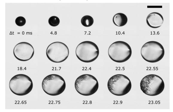
FIG. 7. The growth of the vapor bubble inside an emulsion droplet followed by the wave propagation on the surface of the droplet. The scale bar indicates  $500 \,\mu$ m.
