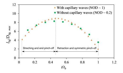
FIG. 11. Evolution of ligament aspect ratio  $(l_{lig}/D_{lig, max})$  following the bubble growth and breakup accompanied by wave propagation and without wave propagation.
