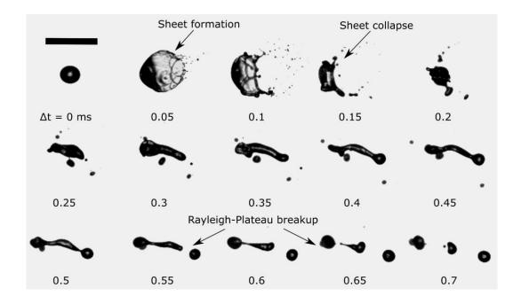
FIG. 15. Crown formation and the breakup of an emulsion droplet ( $D_{onset} \sim 0.2 \text{ mm}$ ) followed by the ligament-mediated breakup. The scale bar indicates 500 µm.
