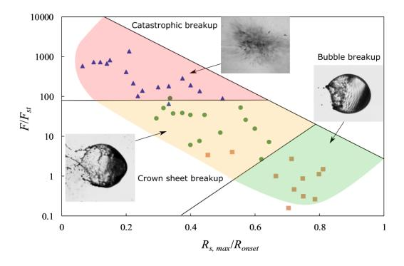
FIG. 19. Overview of the breakup configurations of water-in-fuel emulsions studied in the present work.
