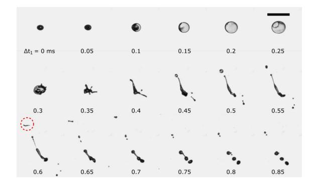
FIG. 13. Vapor bubble growth and breakup without wave propagation on the droplet surface. The red dotted circle indicates the secondary breakup event. The scale bar indicates  $500 \,\mu$ m.
