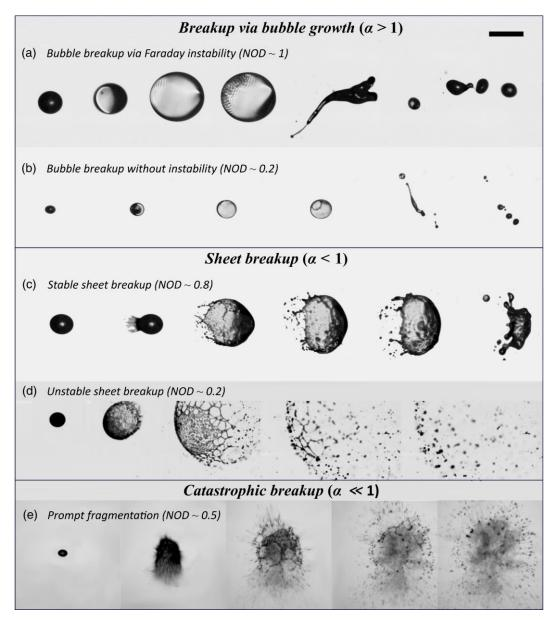
FIG. 5. Modes of fragmentation observed during the evaporation of water-in-fuel emulsion droplets. The scale bar represents 500  $\mu$ m and it is identical across all the sequence of images.
