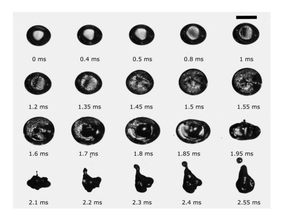
FIG. 14. Formation of a polymer-like structure on the surface of the droplet. The scale bar indicates  $500 \,\mu$ m.
