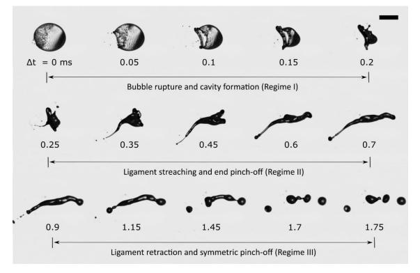
FIG. 10. The rupture of the bubble resulting in the development of long ligament, which consequently undergoes breakup into multiple secondary droplets. The scale bar indicates 500  $\mu$ m.
