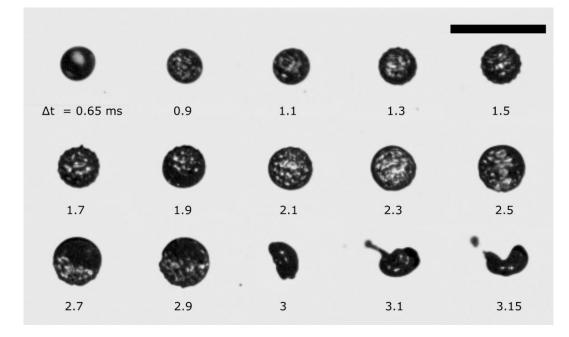
FIG. 12. The growth of the vapor bubble inside the secondary droplet and its subsequent breakup. The scale bar indicates  $500 \,\mu$ m.
