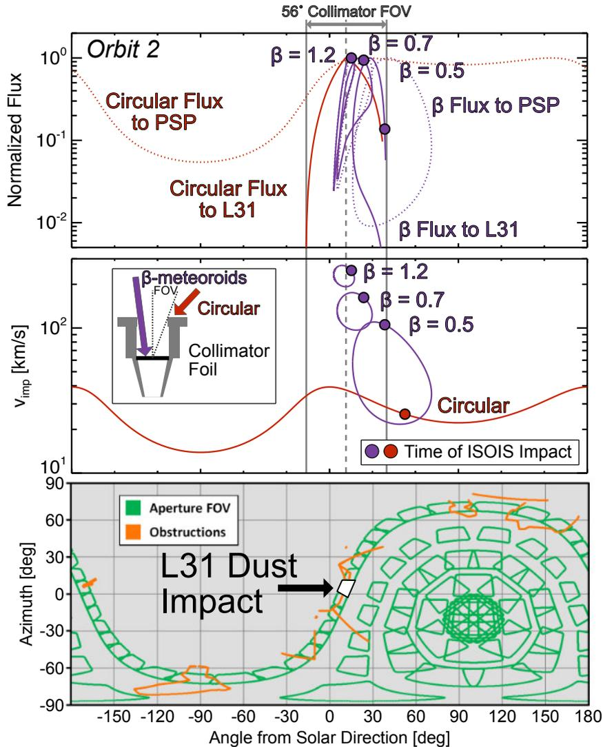
**Figure 9.** Top: normalized flux as a function of impact angle to PSP (dotted) and to the L31 collimator foil (solid) for circular (red) and  $\beta$ -meteoroids (purple). Middle: impact speed as a function of impact angle. Bottom: EPI-Lo aperture FOVs for all 80 look directions, with L31 highlighted.
