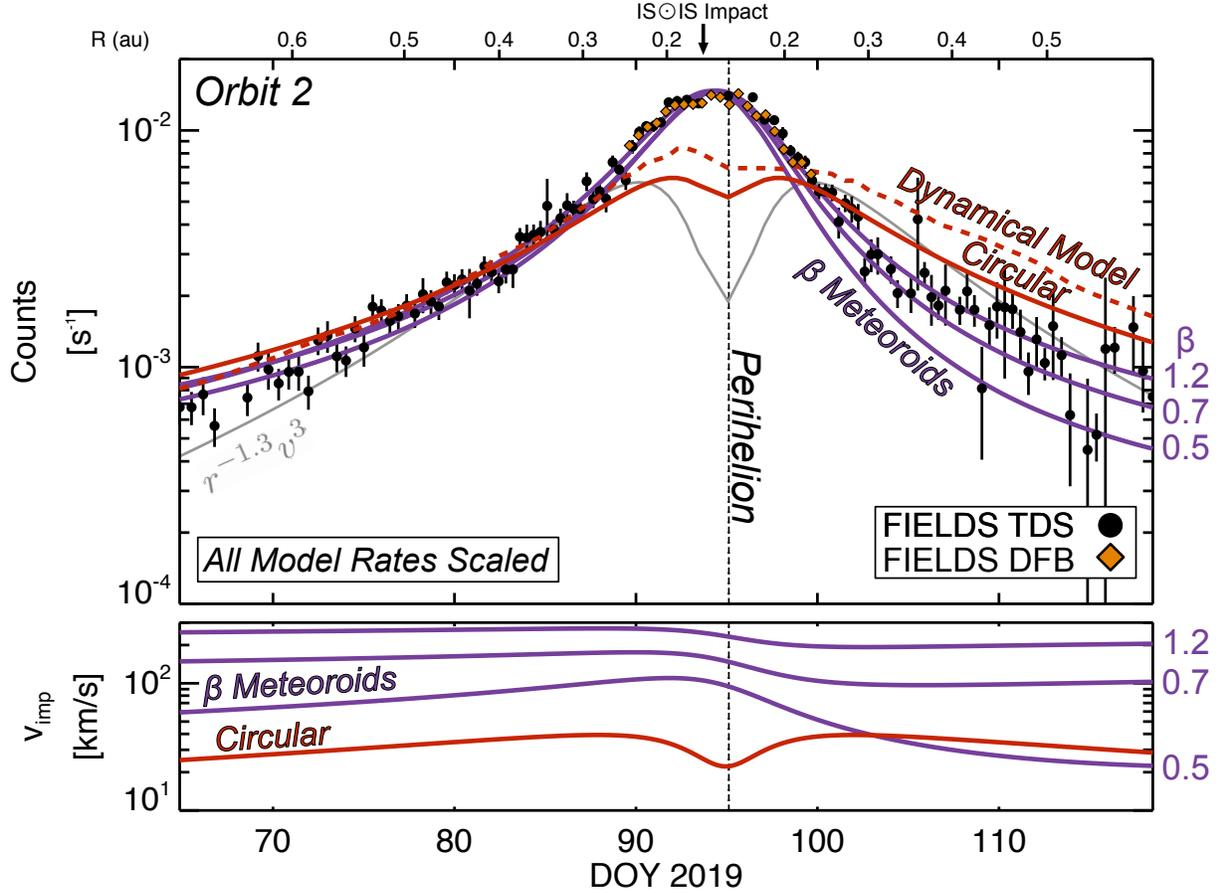
**Figure 7.** Orbit 2 dust summary time series. The top panel shows FIELDs TDS impact rates (black), dynamical model (dashed red), circular model (solid red),  $\beta$ -meteoroids (purple) for  $\beta = [0.5, 0.7, 1.2]$ . The grey line shows a conservative example of an impact rate for a speed-dependent threshold. The bottom panel shows modeled impact speeds for circular (red) and  $\beta$ -meteoroids (purple). The ISOIS dust impact is noted with an arrow just before perihelion.
