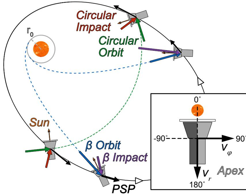
**Figure 1.** Schematic showing vectors for the PSP velocity (black), circular dust velocity vector (green), circular impact velocity (red),  $\beta$  velocity (blue), and  $\beta$  impact velocity (purple) for Orbit 2. The direction to the Sun is shown with the small orange arrows. The inset in the bottom right shows the angle conventions used in this work, in the  $r, \varphi$  coordinate system.
