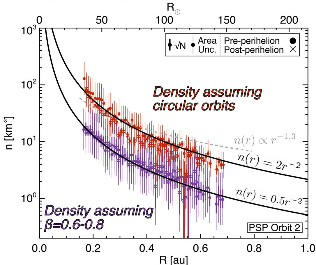
**Figure 8.** Derived dust radial profile from FIELDS-TDS data assuming either all impactors are on circular orbits (red) or  $\beta$ -meteoroids for PSP orbit 2. Thick error bars show Poisson  $\sqrt{N}$  and thin error bars show the range of densities varying the expected area by a multiplicative factor of 2 on top of the Poisson errors.
