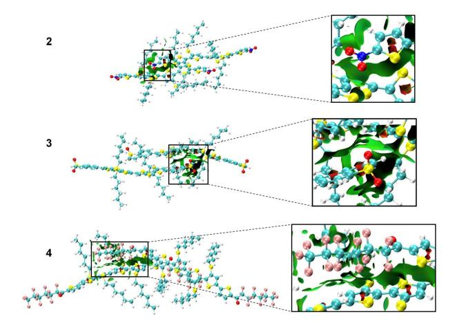
**Figure 5.** NCI indicator isosurface plots for the dimers of compounds 2 (*T4S4TNO2*), 3 (*T4S4TN*) and 4 (*T4S4CF*) identifying hydrogen bonding regions (the green regions between the two molecules). For clarity the isosurfaces were generated only for the regions indicated by the boxes.
