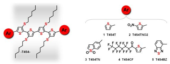
The addition of different terminal Ar groups to the -T4S4- building block allows to obtain a class of Ar-T4S4-Ar oligothiophenes whose electronic distribution is dictated by the Ar groups but that are nevertheless capable to form structurally similar fibers with hierarchical nano- to
