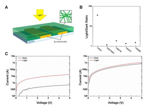
**Figure 9.** A) Device structure for the measurement of the photo-response of the fibers of **1-5** grown on photolithographically-defined gold electrodes on glass, B) Ratio of the conductivities of the materials in the "light" and "dark" conditions. C) Current-Voltage measurements for the fibers of 1 (left panel) and 5 (right panel) grown on photolithographically-defined gold electrodes on glass in the "dark" (black line) and in the "light" (red line) conditions.
