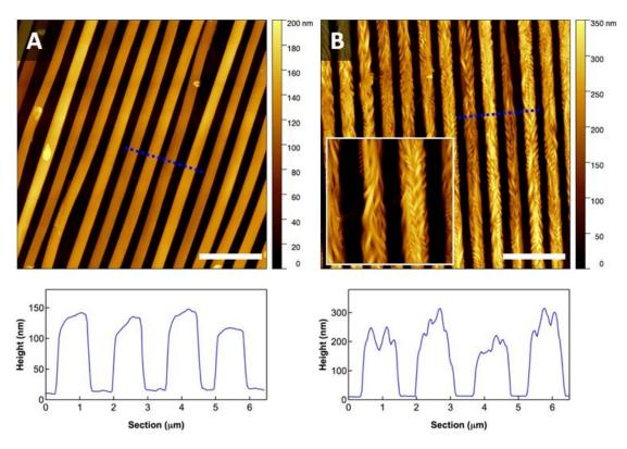
**Figure 2.** AFM images  $20x20 \,\mu\text{m}^2$  and related height plots of the fibers of: (A) **2** (*T4S4TNO2*) and (B) **4** (*T4S4CF*) patterned according the Lithographically Controlled Wetting (LCW)<sup>21</sup> technique. Scale bars =  $5 \,\mu\text{m}$ . Inset image (B): zoom  $5x5 \,\mu\text{m}^2$ .
