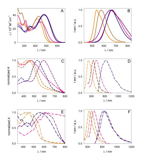
**Figure 3.** Absorption and emission spectra of **1** (*T4S4T*, yellow), **3** (*T4S4TN*, brown), **5** (*T4S4BZ*, pink), 4 (*T4S4CF*, blue) and **2** (*T4S4TNO2*, purple) in different conditions. A-B: air-equilibrated CH<sub>2</sub>Cl<sub>2</sub> at r.t.; C-D: drop-cast films on glass surfaces at r.t.; E-F: as crystalline fibers deposited on glass surfaces at r.t.
