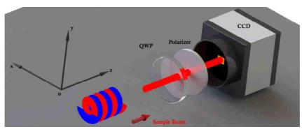
**Figure S1.** Schematic diagram of the characterization system for the Stokes parameters. QWP: quarter-wave plate. The reference systems *oxyz* denotes the laboratory system, and the positive direction of *oz* refers to the propagation direction of the input pulses (denoted by the red arrow).
