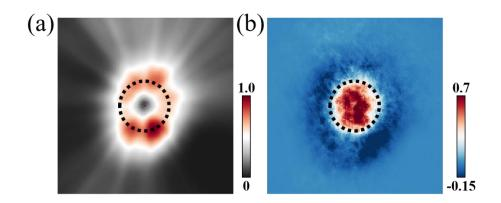
Figure 8. Derived  $S_r$  and  $S_z$  components of the plasmonic SAM, based on the electric field distributions in Figure 7.
