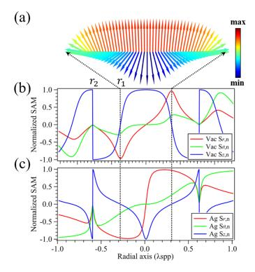
Figure 5. (a) SAM hedgehog profile across the dielectric/metal interface. (b)(c) The radial changes of SAM components in the cylindrical coordinates, in the dielectric and metal sides, respectively.
