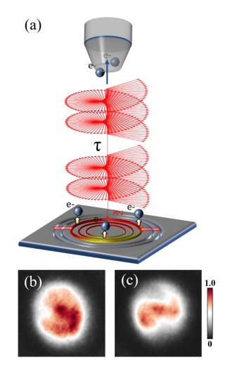
Figure 6. (a) Schematic of the ITR-2P-PEEM experiment. (b)(c) Static, single pulse, PEEM images of an *L*=-1 and *L*=+1 plasmonic vortices. All experimental PEEM image presented have size of  $2\lambda_{spp}$ .
