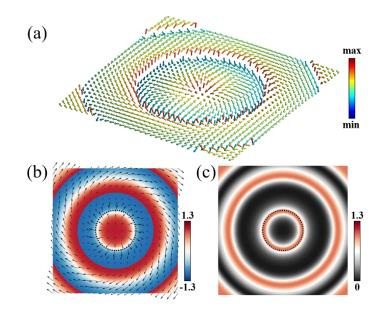
Figure 2. (a) 3D representation of SAM of the plasmonic Skyrmion. (b)  $S_{z,n}$  distribution at the vortex core (color scale). The arrows indicate the directions and amplitudes of the in-plane SAM,  $S_{\parallel,n}$ . (c) Amplitude distribution of  $S_{\parallel,n}$ , which is maximized where the  $E_z$  field is minimized. Dashed circles indicate vortex ring at  $r_1$ .
