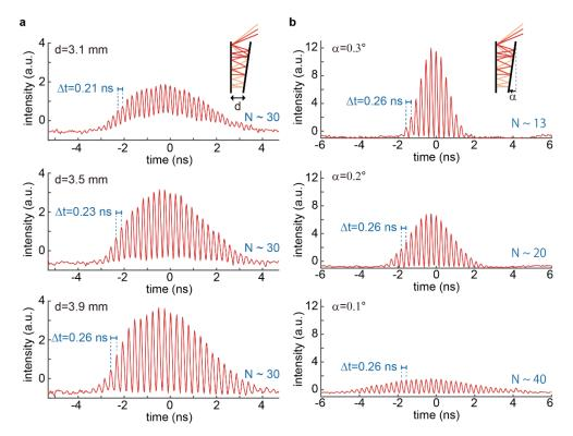
Fig. 2. Characterization of a time-stretched MIR pulse. a Mirror-pair-distance (*d*) dependence on the temporal interval of the sub-pulses ( $\Delta t$ ). b Mirror-pair-angle ( $\alpha$ ) dependence on the number of sub-pulses (*N*).
