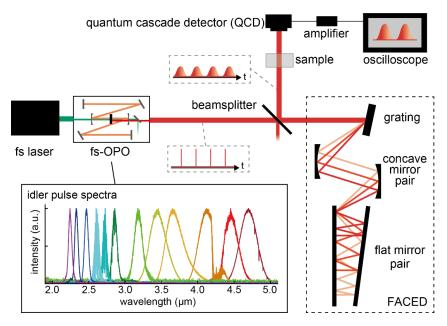
**Fig. 1. Schematic of TS-IR spectrometer.** The MIR fs pulse is stretched in the FACED system and detected by the QCD after passing through the sample. The QCD signal is amplified and digitized with the fast oscilloscope. The bottom left inset shows the wavelength-tunable spectra of the idler pulses generated by the fs-OPO.
