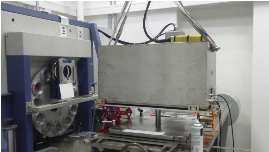
Figure 1: Free-air ionization chamber placed in front of the X-ray generator on the positioning table and ready for the measurement. Connected cables and the voltage divider box are visible on the rear panel.
