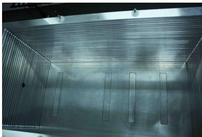
Figure 7: View into the inner chamber to collecting electrodes (HV electrode removed).
