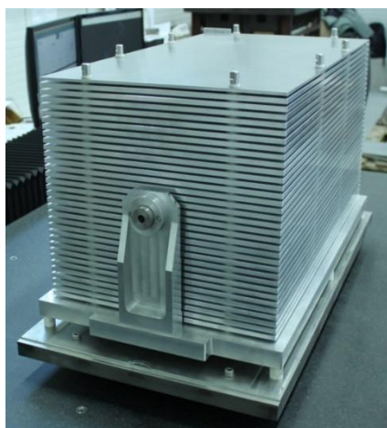
Figure 6: Completed free-air chamber (without outer case). In front: cylindrical tungsten aperture in its holder.
