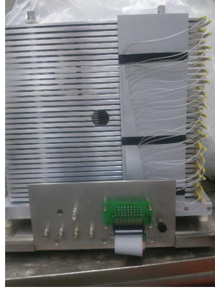
Figure 9: Back wall of the chamber with the voltage divider and connectors for high voltage and measurement of ionizing current (outer case removed).
