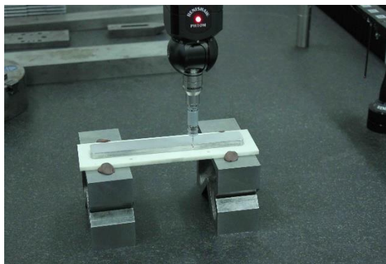
Figure 5: Measurement of collecting electrode dimensions using CMM.
