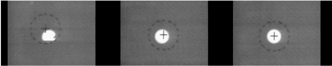
Figure 10: Iterative procedure of FAC alignment: The dashed circle represents the rear opening of FAC, the bright circle is the visualised front opening. Goal is to align these two circles.
