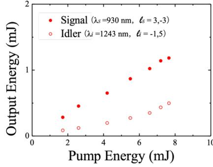
Fig. 3 Power scaling of the 930 nm signal and corresponding 1243 nm idler outputs.
