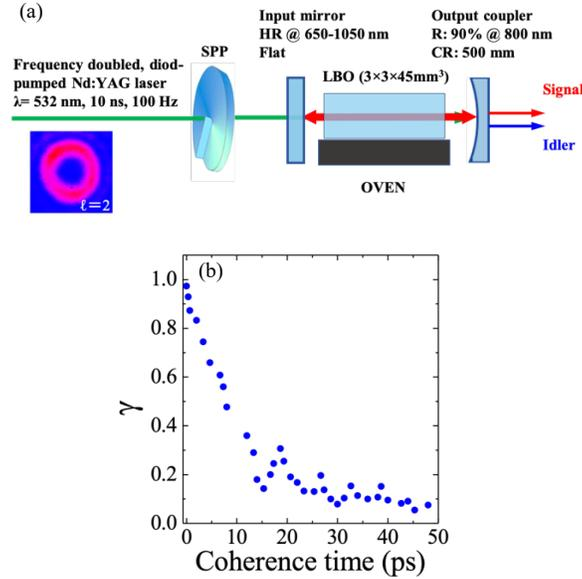
Fig. 1(a) Experimental setup of singly resonant optical parametric oscillator. (b) Measured temporal coherence of pump laser.
