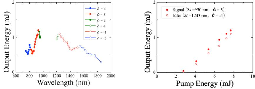
Fig. 7. Tunability and power scaling of signal and idler outputs.
