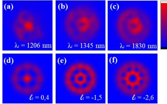
Fig. 4(a-c) Wheel-shaped idler modes with  $\ell_i=0$  & 4, -1 & 5, and -2 & 6. (d-f) Theoretical wheel-shaped idler outputs.
