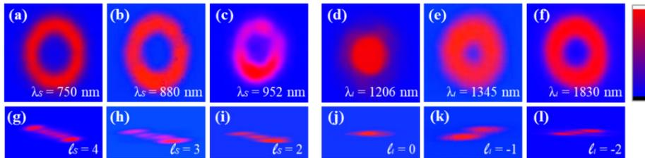
Fig. 6 Spatial profiles of (a–c) signal (750 nm, 880 nm, and 952 nm) and (d–f) idler (1830 nm, 1345 nm, and 1206 nm) vortex outputs. Inclined focused spatial forms of (g–i) signal (770 nm, 880 nm, and 952 nm) and (j–l) idler (1830 nm, 1345 nm, and 1206 nm) outputs.
