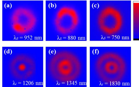
Fig. 9 (a-c) Ring-shaped modes with  $\ell_s = \pm 2, \pm 3, \text{ and } \pm 4$ . (d-f) Double-ring modes with  $\ell_r = -4$  and 0, -3 and 1, and -2 and 6.
