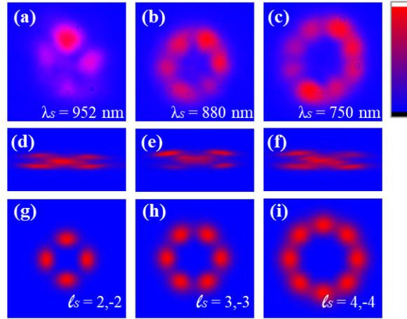
Fig. 2 (a–c) Flower modes with  $\ell_s = \pm 2, \pm 3$ , and  $\pm 4$ . (d–f) Wavefront measurement of signal outputs with a tilted lens. (g–i) Theoretical flower modes with  $\ell_s = \pm 2, \pm 3$  and  $\pm 4$ .  $\alpha$  is 0.32.
