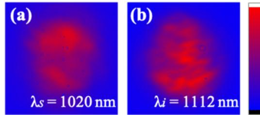
Fig. 8(a) 1020 nm signal and (b) corresponding 1112 nm idler outputs from the double resonance region.
