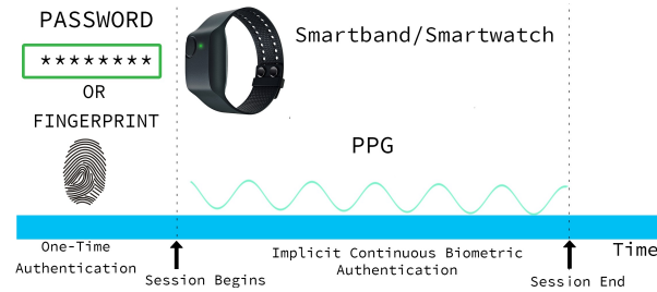
Fig. 3. Our proposed solution continuously authenticate the user by processing the RR intervals coming from the smartband.
