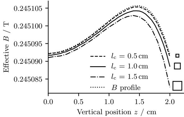
Fig. 9. Simulation results for determination of the  $B$  profile for different coil side lengths. A square coil cross section was used for the simulations. The coil cross section is shown on the right hand side.
