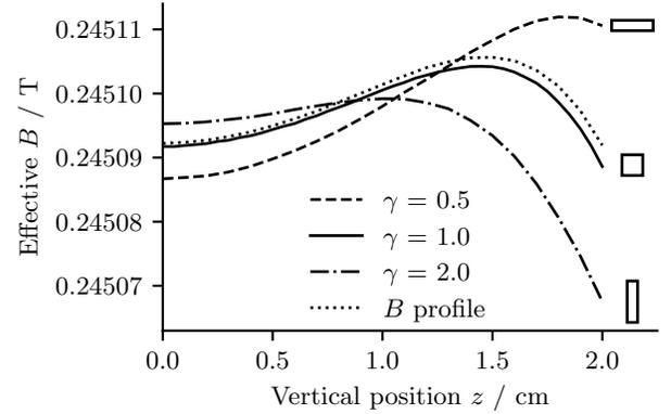
Fig. 10. Influence of the aspect ratio in the  $B$  profile. For these simulation results a coil with cross section area of  $1 \text{ cm}^2$  was used. The coil cross section is shown on the right hand side.
