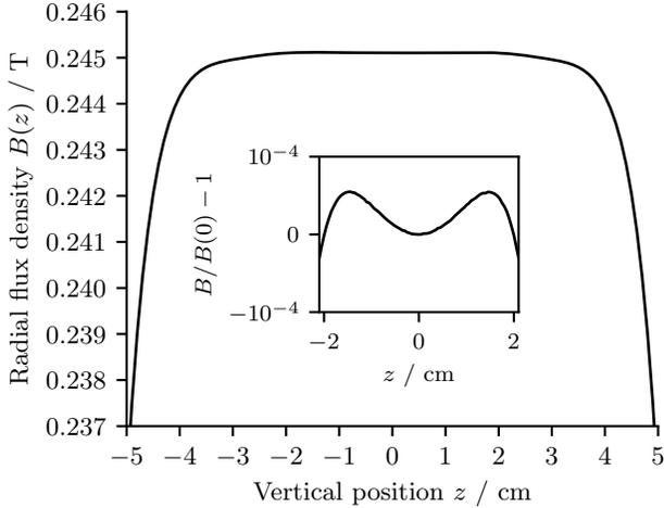
Fig. 6. Profile for the radial magnetic flux density  $B$ . The box inside the plot shows the profile deviation for the precision air gap of 4 cm. This profile was obtained by using finite element analysis.
