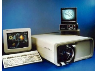
Fig. 3. WYKO-6000 Fizeau interferometer. The B&W video-monitor at top, allows real-time fringe visualization. The computer, the CCD-camera, and fringe-software were upgraded.
