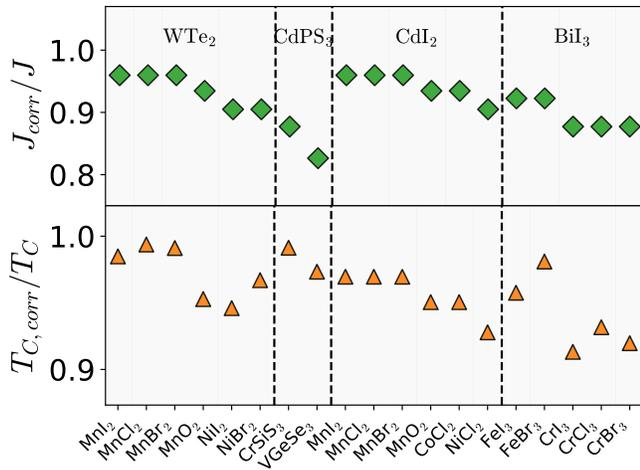
FIG. 3. Corrections to exchange parameters (top panel) and Curie temperatures (lower panel) obtained with PBE+U for all insulating ferromagnets with positive values of  $\Delta$  present in the C2DB.
