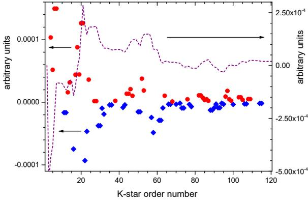
FIG. 10: Individual  $K$ -star contributions to electric field gradient at  $T = 300$  K [each term  $\propto j_2(KR_{MT})S_Q(\hat{K})(\langle\rho(\vec{K})\rangle_{T=300} - \langle\rho(\vec{K})\rangle_{T=0})$ , Eq. (23)]. Blue diamonds - negative contributions, red circles - positive contributions, dashed purple curve - sum of all contributions up to the chosen  $K$ -star. The final value of the sum (at  $n \geq 120$ ) is positive, which leads to an increase of  $V_{zz}$  at 300 K.
