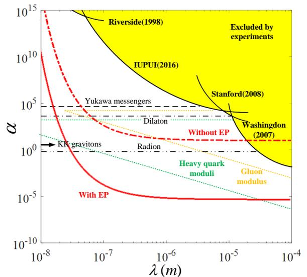
FIG. 5. Experimental constraints of short-range forces caused by Yukawa-type interaction potentials [19-22] and theoretical predictions of this work. The shaded region is excluded with 95% confidence level. The full line and dashed denote the results of EP measurement scheme and conventional optomechanical sensor respectively.
