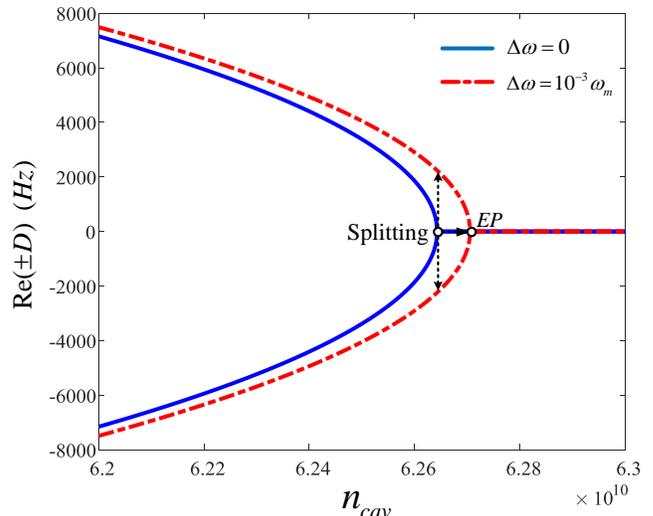
FIG. 3. Eigenfrequency difference of the effective mechanical system before perturbation (full blue lines) and after perturbation (dashed red lines) by variation of force gradient corresponding to a frequency shift of  $\Delta\omega = 10^{-3}\omega_m$ .
