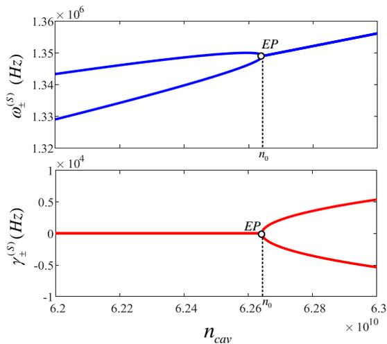
FIG. 2. Real(left) and imaginary(right) part of the mechanical eigenfrequency as a function of  $n_{cav}$  with  $\Delta = \omega_m$ .
