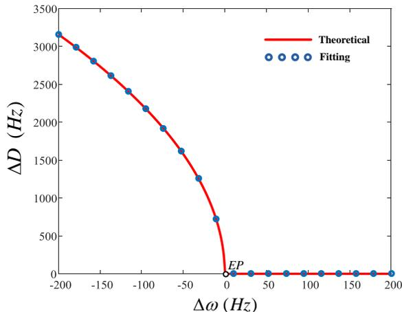
FIG. 4. Theoretical and fitting curves of super mode frequency splitting as a function of perturbation. The fitting expression is Eq.(15) with  $Y = 5 \times 10^4$ .
