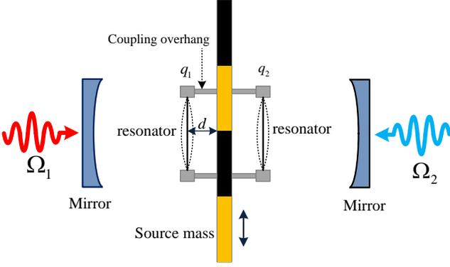
FIG. 1. Generic setup. A coupled cavity optomechanical system with double resonators. A source mass with varying density sections is positioned in the middle. The two cavities are driven by blue- and red-detuned laser, respectively.
