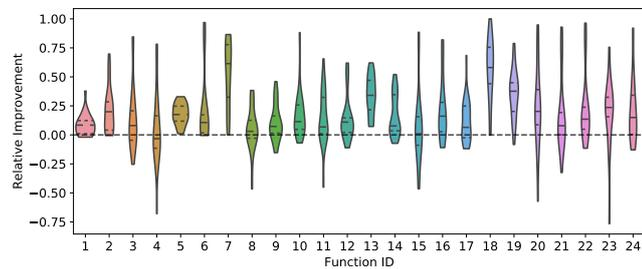
**Figure 5:** Distribution of relative improvement in ERT between the default and tuned hyperparameters. For each function, 30 variants are tuned with MIP-EGO, and the resulting (variant, hyperparameters)-pairs are rerun 250 times to validate the results. The same is done for the default hyperparameters, and then the relative improvement in ERT is calculated.
