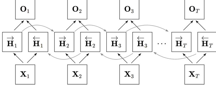
Figure 2: Architecture of a bidirectional recurrent neural network
