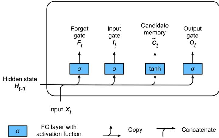
Figure 9: Computation of candidate memory cells in LSTM: [24]
