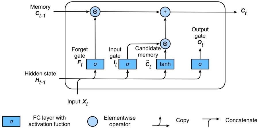
Figure 10: Computation of memory cells in an LSTM: [24]
