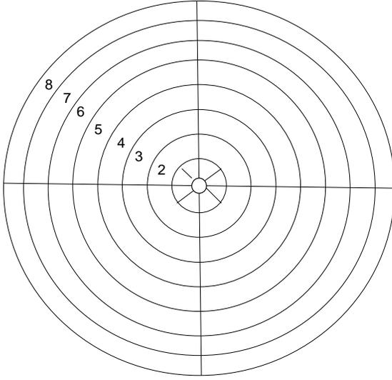
**Fig.2.** TPC anode structure.
