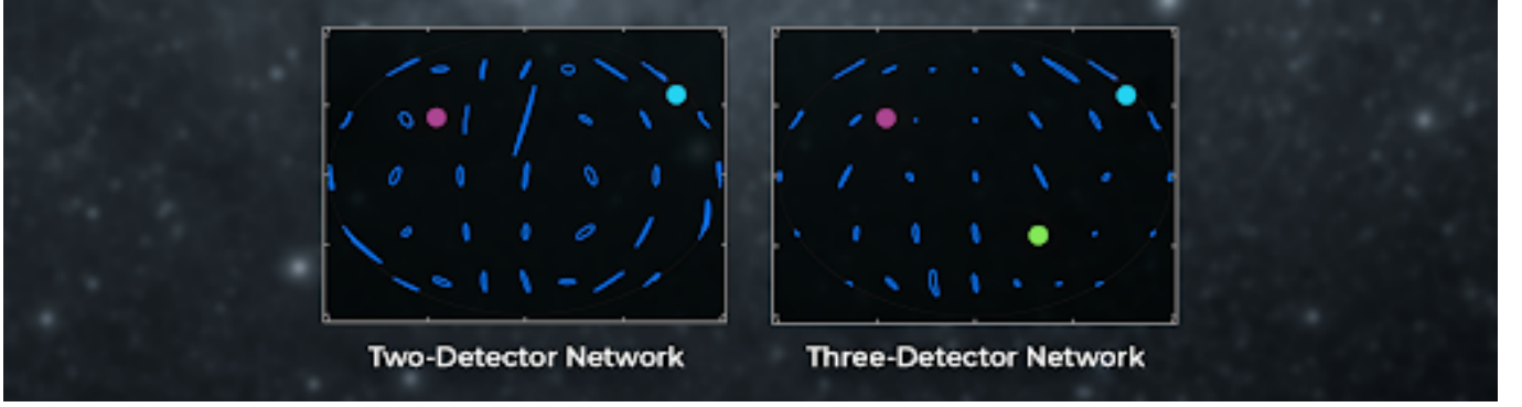
FIG. 1: Gravitational-wave sky maps (adapted from [19]). The left-hand side shows the localisation provided by a two-detector Cosmic Explorer network (for a binary neutron star merger located at a redshift of z=2 ) while the right-hand side shows the improved localisation made possible with a three-detector network. Each blue ellipse is a localisation region for a different binary merger. The filled-in circles represent the locations of gravitational-wave observatories in a global network: Europe (purple), USA (cyan), and Australia (green). Each year, the three-detector network will localise over a thousand binary neutron stars to better than one square degree.
