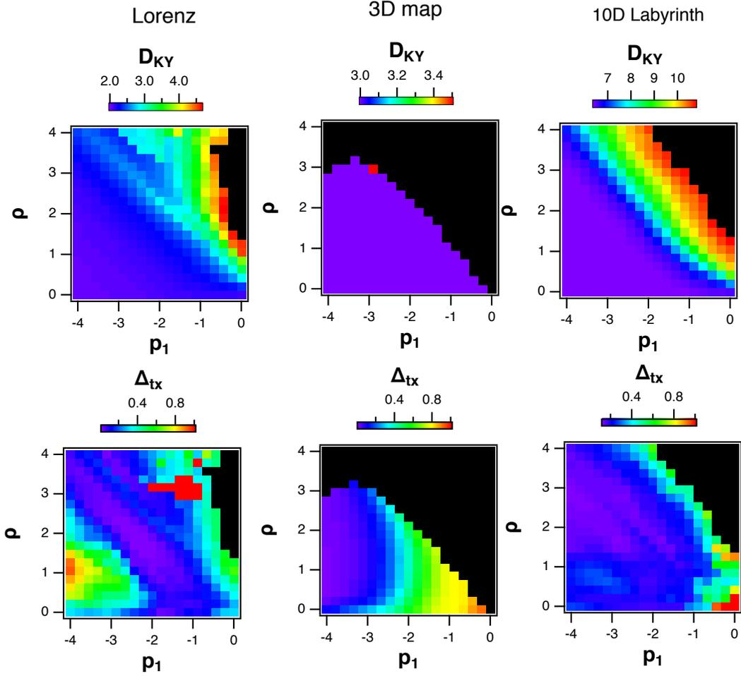
FIG. 8: Results for the polynomial nodes. The top plots are the Kaplan-Yorke dimension  $D_{KY}$  for the polynomial reservoir driven by the Lorenz  $x$  signal, the 3d map signal, or the 10d Labyrinth signal, as the spectral radius  $\rho$  and parameter  $p_1$  vary. The bottom plots are the training error  $\Delta_{tx}$  for the same three combinations. The black regions correspond to a positive Lyapunov exponent for the reservoir.
