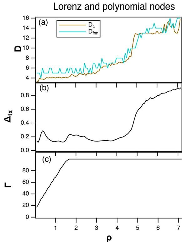
FIG. 4: (a) Covariance dimension  $D_c$  and false nearest neighbor dimension  $D_{fnn}$  of a reservoir consisting of 100 polynomial nodes driven by the Lorenz  $x$  signal. The parameters were indicated in section VII. As the spectral radius  $\rho$  increases, both the covariance and false nearest neighbor dimensions increase. (b) Testing error  $\Delta_{tx}$  for predicting the Lorenz  $z$  signal from the Lorenz  $x$  signal. (c) Covariance rank as defined in eq. (12).
