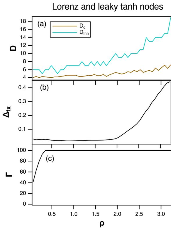
FIG. 5: (a) Covariance dimension  $D_c$  and false nearest neighbor dimension  $D_{fnn}$  of a reservoir consisting of 100 leaky tanh nodes driven by the Lorenz  $x$  signal. As the spectral radius  $\rho$  increases, both the covariance and false nearest neighbor dimensions increase. (b) Testing error  $\Delta_{tx}$  for predicting the Lorenz  $z$  signal from the Lorenz  $x$  signal. (c) Covariance rank as defined in eq. (12).
