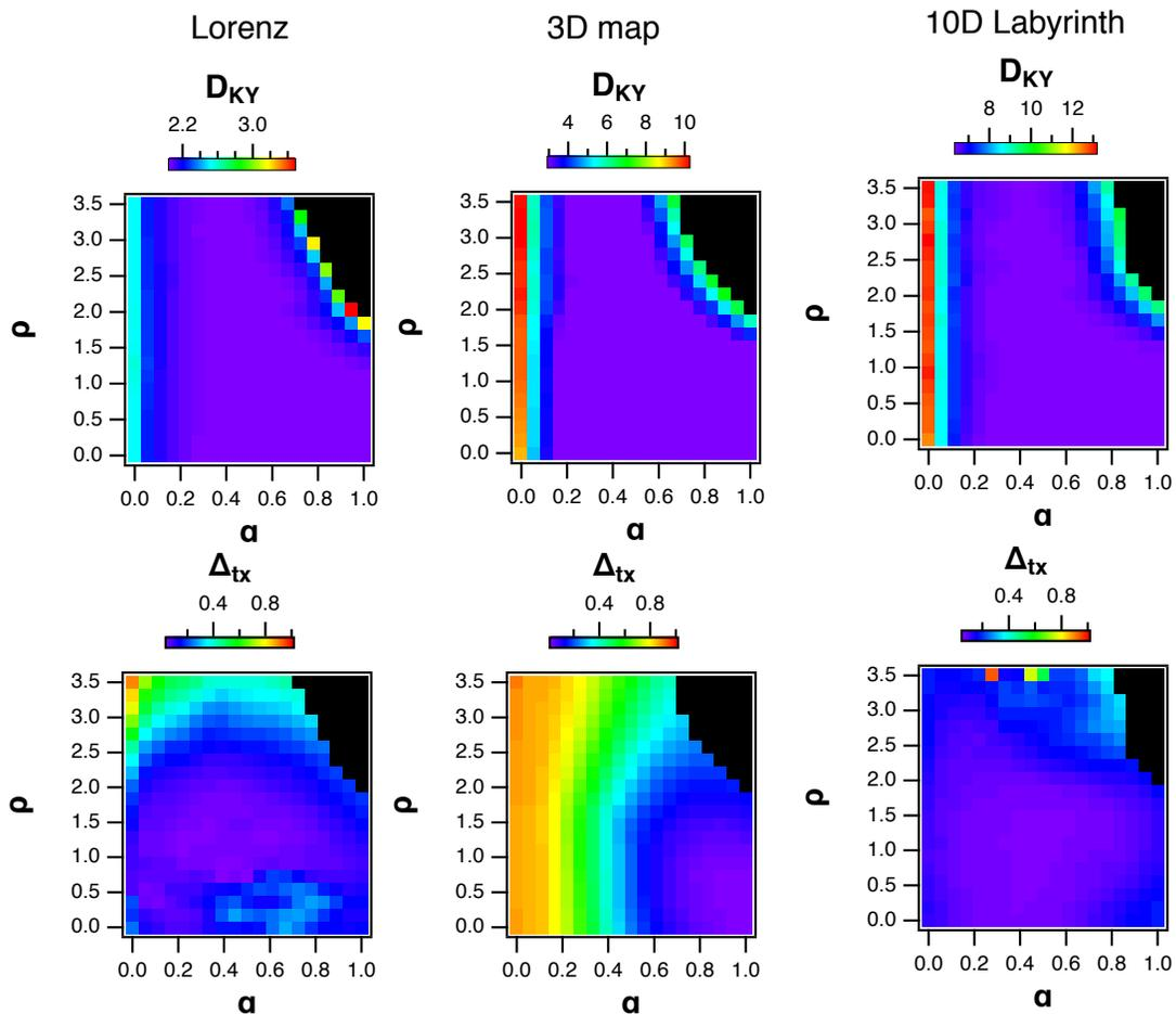
FIG. 9: Results for the leaky tanh nodes. The top plots are the Kaplan-Yorke dimension  $D_{KY}$  for the polynomial reservoir driven by the Lorenz  $x$  signal, the 3d map signal, or the 10d Labyrinth signal, as the spectral radius  $\rho$  and parameter  $p_1$  vary. The bottom plots are the training error  $\Delta_{tx}$  for the same three combinations. The black regions correspond to a positive Lyapunov exponent for the reservoir.
