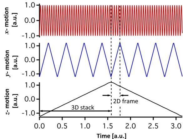
Figure 2: Sketch of the synchronized motion of the scanning units in the case of the standard 3D mode. The resonant mirrors perform a sinusoidal motion, scanning two lines per period of motion. To minimize dead time, the y- and z-motion is rectilinear and scanned also in a bidirectional way. The number of lines per 2D frame and the number of 2D frames per 3D stack is adjustable through the frequencies chosen to drive the galvanic mirrors and the  $z$  motion of the focus.
