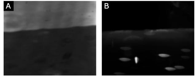
Figure 8: Synchronized confocal (A) and astigmatic (B) measurements of a moving three phase contact line.
