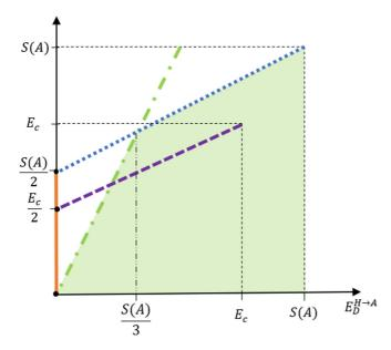
FIG. 5. Upper bounds on quantum key repeater rates. Dotted blue line: introduced here in eqn. (20), solid orange line: special case for  $I_{\rm coh} = 0$ , dashed violet line: [15], and dotted-dashed green line: only for some states [19]. Shaded region corresponds to a combination of bounds.
