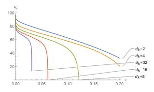
FIG. 12. Plots of lower bound on percentage of memory overhead from theorem 5, with different values of  $d_k$ .
