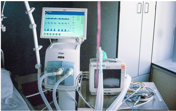
Figure 19: User interface for monitoring a patient’s vital functions. A monitor is combined with an auditory display to serve as a multi-modal user interface.
