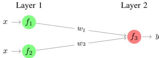
Figure 10: A synthetic computer system where  $f_1$  and  $f_2$  are two computer models with a common one-dimensional input but different scalar-valued outputs, and  $f_3$  is a computer model with two-dimensional input and one-dimensional output.
