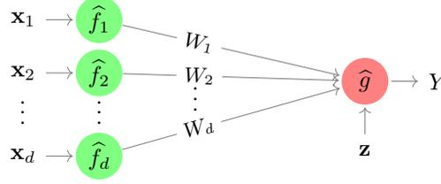
Figure 1: The connections of emulators to be linked for emulating a two-layered computer system.  $\hat{f}_1, \hat{f}_2, \dots, \hat{f}_d$  are one-dimensional emulators approximating  $d$  outputs from computer models in the first layer;  $\hat{g}$  is a one-dimensional GaSP emulator approximating a scalar-valued output of the computer model  $g$  in the second layer of the system.
