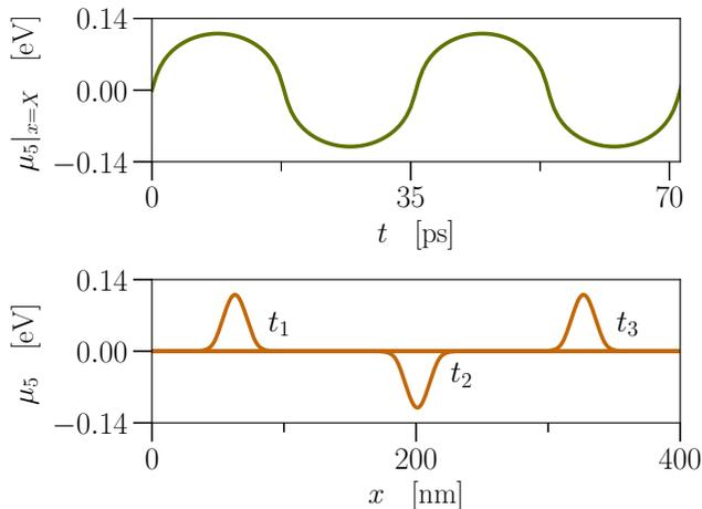
FIG. 2. Axial chemical potential  $\mu_5$  as function of time  $t$ , evaluated at the domain wall center  $x = X(t)$  (upper panel) and as a function of  $x$  at times  $t_1 = 100\tau_\phi + \tau_\phi/4$ ,  $t_2 = 320\tau_\phi - \tau_\phi/4$  and  $t_3 = 520\tau_\phi + \tau_\phi/4$  (lower panel). Here we take chemical potential  $\mu = 10$  meV, temperature  $T = 300$  K and magnetic field  $B = 1$  T; other parameters are given in [28].
