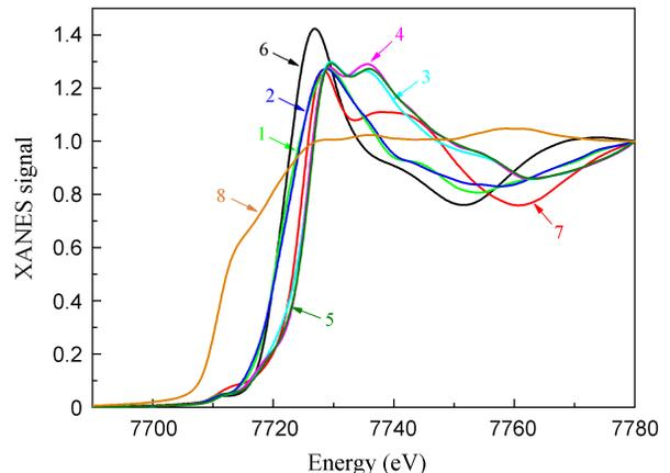
FIG. 2. XANES spectra of five  $\text{SrTiO}_3(\text{Co})$  samples and three reference compounds. (1) Co2A1600, (2) Co2A1500, (3) Co2A1100, (4) Co3B1500, (5) Co3B1100, (6)  $\text{Co}(\text{NO}_3)_2 \cdot 6\text{H}_2\text{O}$ , (7)  $\text{LaCoO}_3$ , (8) Co metal foil.
