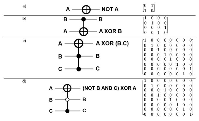
Figure 5 a) NOT gate b) CNOT gate c) Toffoli gate with two positive controls d) Toffoli with one negative control and one positive control
