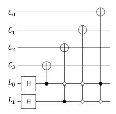
Figure 9 A quantum image circuit.
