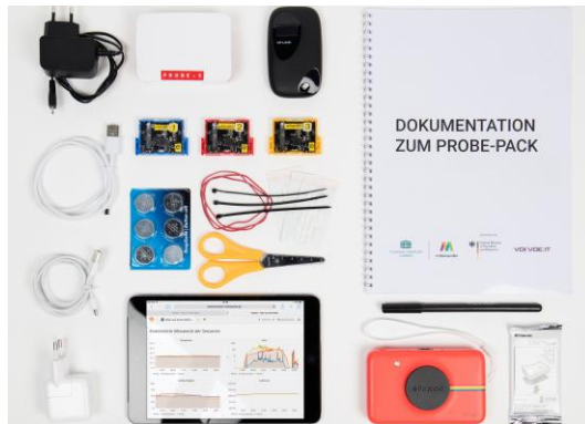
Figure 4: Components of the Sensing Home kit (SensorTags, Raspberry Pi, tablet pc, etc.) .
