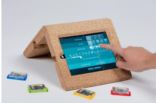
Figure 7: Sensorstation input screen side and color-coded SensorTags.
