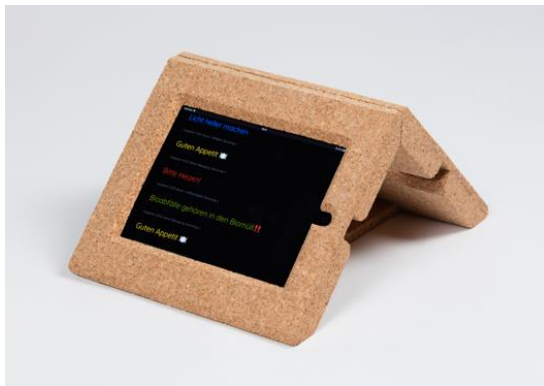
Figure 8: Sensorstation output screen side with message stream. The notifications are time-stamped and color-coded according to the assigned SensorTag.
