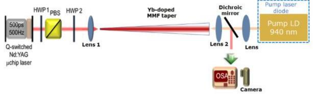
Fig. 1. Schematic of the experimental setup for coupling microchip laser pulses at 1064 nm as well as a CW pump laser diode (LD) into the Yb-doped MMF taper.
