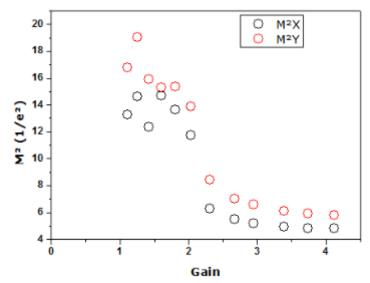
Fig. 6. Measured beam quality M<sup>2</sup> parameter versus laser gain, for the case of Fig. 5.
