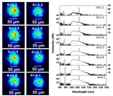
Fig. 5. Left panels: Near-field spatial beam distribution from the largest core diameter face of the 5 m long taper, with 10 kW input power at 1064 nm, and different values of gain G; Right panels: corresponding spectra versus gain G.
