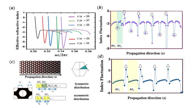
Figure 5. Computed results (a) effective refractive index for different radii values in an hexagonal lattice (b) extracted refractive indexes for symmetric hexagonal lattice in both first and second Brillouin zones for different radii values with ascending orders through the propagation direction (c) All details of proposed lattice in two types of distributions (symmetric and asymmetric) in which the asymmetric distribution without experiencing the second Brillouin zone traverses to
