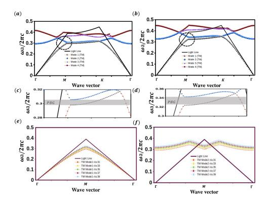
**Figure 2.** Swinging band diagram for a hexagonal lattice for the under study lattice (a) with the radii equals to 0.31 PBG occurs around 0.3 in  $\Gamma - M$  direction (b) with the radii equals to 0.39 PBG occurs around 0.33 in  $\Gamma - M$  direction (c), (d) zoomed in part of the photonic band gaps (e) swinging first band to the upper angular frequencies with increasing the radii (f) swinging second band to the higher angular frequencies with the increasing radii
