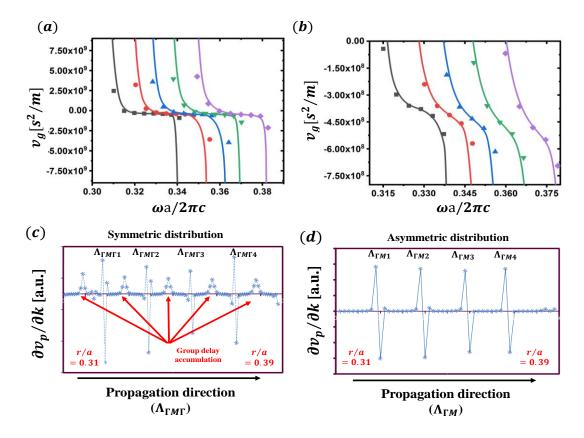
Figure 6. (a) Group velocity with swinging radii from 0.31 (black) to 0.39 (pink) (b) and its zoomed in region with negative group velocity (c) symmetric distribution which accumulate group delay in each transition from first Brillouin zone to the second one and weak compensating for transition of perturbing radii (b) asymmetric distribution with smooth group delay and compensating group delay in each transition of perturbing radii
