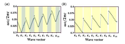
Figure 4. Dispersion diagram in asymmetric cluster (hexagonal lattice) through the light path of the modulated optical element (a) Discrete portion of band diagram in the first Brilouin zone of entire lattice (b) Gradient of wave vector in reciprocal space with continuous broken symmetries of lattice
