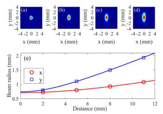
Fig. 3. THz beam profile measurement results of the LN TPA. (ad) are THz beam profiles measured at 2.0, 5.0, 8.0, and 11.0 mm downstream the THz radiation exit surface (S2) of the LN crystal. (e) plots the beam radii for THz beam as a function of the measurement distance. The solid curves were calculated according to the estimated  $M^2$  parameters.
