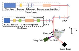
Fig. 1. A sketch of the TPA experimental setup.
