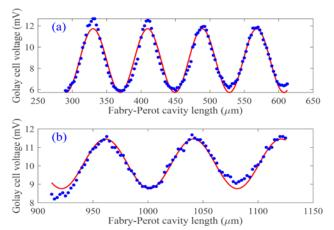
Fig. 2. Measurement result for THz radiation wavelength (a) and bandwidth (b).
