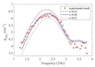
Fig. 5. THz parametric gain  $(g_{THz})$  vs frequency. The curves represent theoretical results calculated using Eq. (3), for which 3 different  $\kappa$  values were used.
