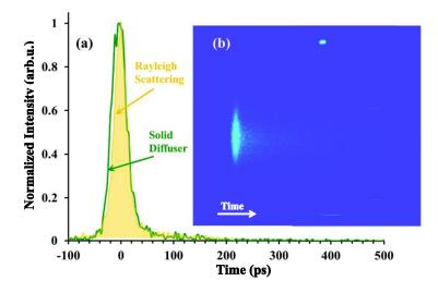
**FIG B.** (a) In yellow: the reference pulse obtained by sending the laser beam through a dispersed mist. Green: reference pulse obtained with a solid diffuser surface. The dashed line indicating the center of gravity of the yellow reference will be used as the time of arrival of the fs pulse. (b) typical streak camera image frame.
