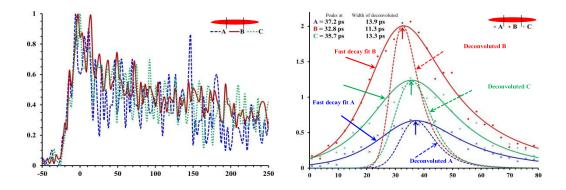
**FIG.3** Left : Integrated IR emission from selected spatial regions of the plasma labeled as "A", "B" and "C" as shown in the inset. Right: Comparing fast decay and built up time of the emission at 391 from the same selected regions.
