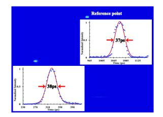
**FIG A:** Typical average of 1000 frames, recording the scattering of a diffuser. For ideal resolution, the reference (top) and the image have the same intensity. Note that they also have the same width.
