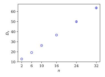
Fig S1. The separation distance,  $D_s$ , as a function of the number of spacers estimated from the first peak of the pair correlation function, g(r), from molecular dynamics self-assembly simulations.
