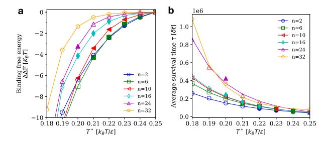
*Figure 4.* (a) DFP binding free energy  $\Delta\Delta F$  as a function of temperature for a different number of spacers n. The filled symbols highlight the systems forming an FCC lattice, while the open symbols show the systems forming disordered structures. (b) Average strand survival time
