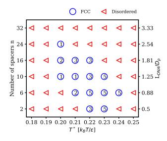
*Figure 3.* Crystallization order diagram as a function of temperature, T<sup>\*</sup>, and the number of spacers, n. Blue circles and red triangles represent the conditions for identifying FCC and disordered structures, respectively. Indices in blue circles show the number of simulations forming FCC lattice from 5 parallel simulations. The second y-axis on the right shows the
