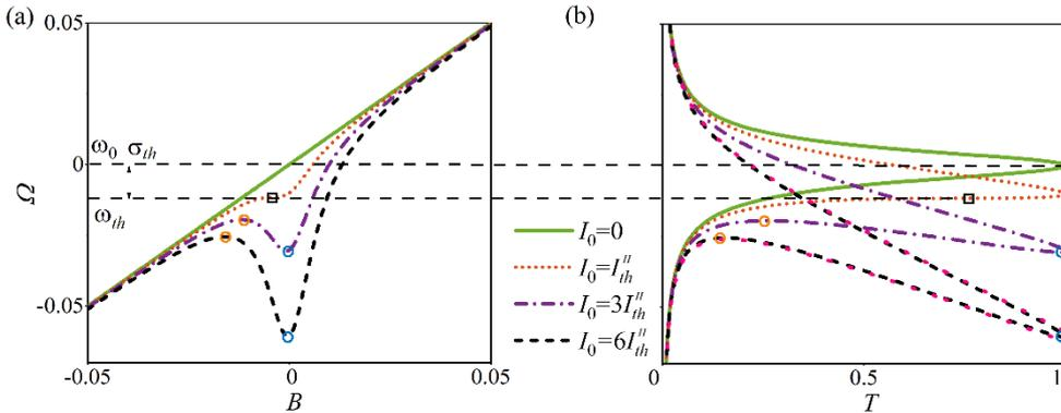
Fig. 3. Fragments of the nonlinear dispersion characteristic (a) and the frequency response (b) for the various input intensities.
