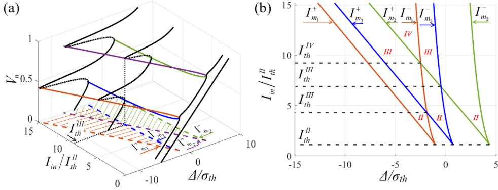
Fig. 7. Nonlinear surfaces of the normalized value  $V_n$  as a function of the normalized intensity and frequency detuning showing the multistability in the two-RC circuit (a) and projection of this surface onto a plane  $(I_0/I_{th}^{II}, \Delta/\sigma_{th})$  showing the multistability in the three-RC circuit (b).
