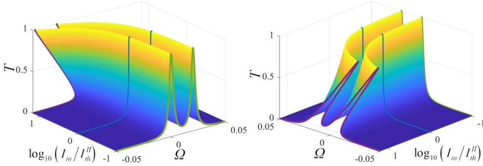
Fig. 6. Color-mapped nonlinear response surfaces for the two-RC resonant circuit calculated for the various intensities and shown for the different viewing angles.
