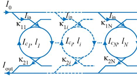
Fig. 5. Schematic of the multi-ring resonant circuit.
