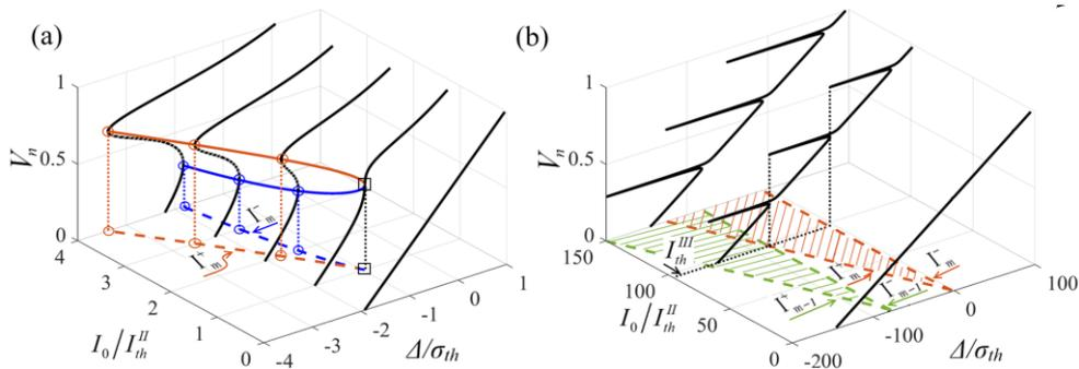
Fig. 4. Nonlinear surfaces of the normalized value  $V_n$  as a function of the normalized intensity and frequency detuning showing bistability (a) and tristability regimes (b).
