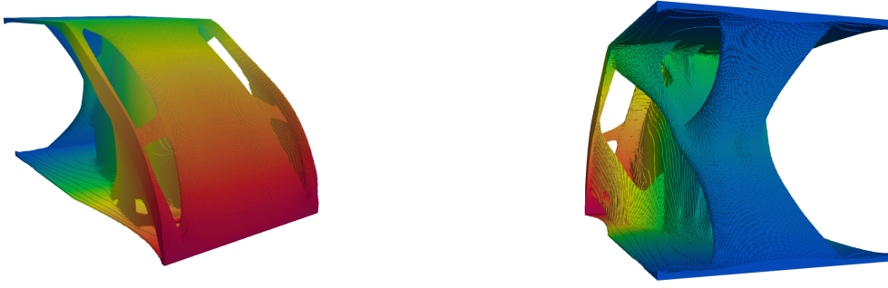
Fig. 15: Optimized structure for 3D cantilever beam problem at an increased resolution.
