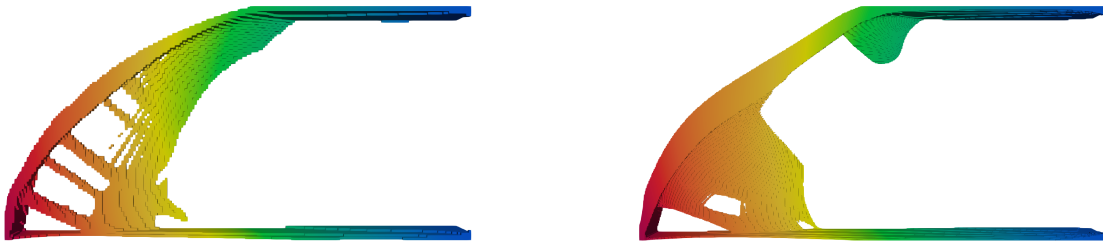
Fig. 17: Comparison of structure along lateral edge of domain at coarse (left) and fine (right) resolution.
