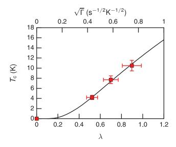
FIG. 3. Superconducting transition temperature  $T_c$  vs.  $\sqrt{\Gamma}$ , where  $\Gamma$  is the strength of spin fluctuations just above  $T_c$  for  $H_{\parallel a}$  in Co-doped FeSe single crystals. The solid line represents our theory of  $T_c$  vs. the coupling constant  $\lambda \propto \sqrt{\Gamma}$  (see text). The error bars represent the uncertainty in determining  $T_c$  and  $\Gamma$ .
