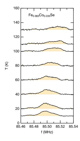
Supplementary Figure 1. Temperature dependence of <sup>77</sup>Se spectrum at 3.6%Co doping. The full-width-at-half-maximum (FWHM) significantly increased at this doping. Since the splitting of the line due to nematicity is smaller than the FWHM,  $T_{\text{nem}}$  cannot be identified.
