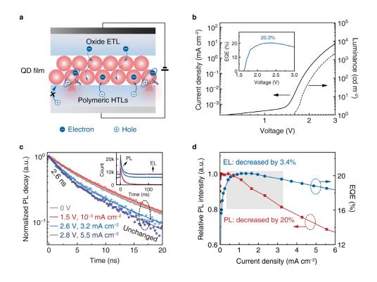
Fig. 4: Exciton generation in a high-efficiency QD-LED.
