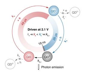
Fig. 3: Dynamics of the single-dot EL cycle.
