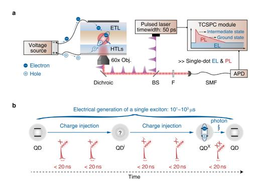
Fig. 1: Electrically-pumped single-nanocrystal spectroscopy.
