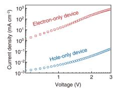
**Supplementary Figure 10: Current densities versus voltages of an electron-only device and a hole-only device.** The structure of the electron-only device is ITO/QDs (25 nm)/Zn<sub>0.9</sub>Mg<sub>0.1</sub>O (65 nm)/Ag. The structure of the hole-only device is ITO/PEDOT:PSS (40 nm)/TFB (45 nm)/QDs (25 nm)/MoO<sub>3</sub> (5 nm)/Au.
