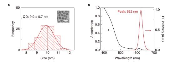
**Supplementary Figure 1: The CdSe-CdZnS QDs. a** Size distribution histogram of the CdSe-CdZnS QDs. Inset: a typical TEM image (scale bar: 20 nm). **b** Ultraviolet-visible absorption and PL spectra of the solution of QDs in octane.
