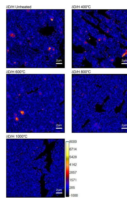
Figure 3. Representative NanoSIMS  $\delta D$  ion images of the different samples. Hotspots are clearly visible in the samples heated up to 600 °C, but are essentially gone in the sample heated to 800 °C and above.
