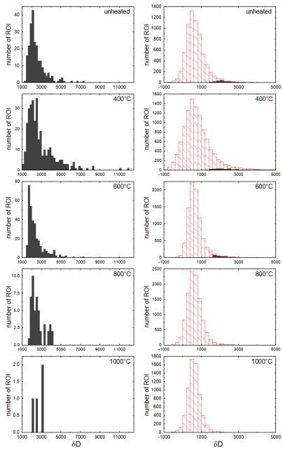
Figure 4. Histograms showing the distribution of  $\delta D$  values in anomalous ROIs (left) and of all ROIs as well as anomalous ROIs (right) for the different samples. The distribution of all ROIs, as well as those of the anomalous ROIs, become narrower with increasing peak heating temperature.
