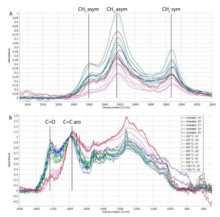
Figure 5. FTIR spectra of the samples normalized to an absorbance of 1 at 1600 cm<sup>-1</sup>, the C=C stretch peak position in the unheated sample. (A) The aliphatic stretching region  $3050-2800 \text{ cm}^{-1}$ . (B) The spectra in region  $1900-750 \text{ cm}^{-1}$ . The relative decrease in the intensity of the C=O peak is clearly seen.
