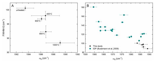
Figure 2. The Raman G-band parameters for the Cold Bokkeveld IOM heated to different temperatures. The G-band peak width (FWHM) becomes narrower with increased heating and there is a tendency for the G-band peak position (🛛) to move towards higher wavenumbers. (B) The data in this study compared to the range of G-band parameters determined for IDPs by Busemann et al. (2009).
