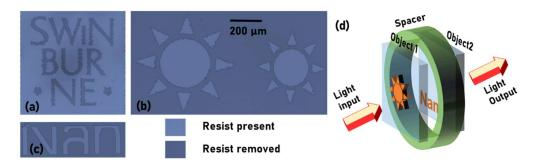
**Figure. 3** Optical microscope images of (a) Swinburne logo, (b) two stars and (c) object 'Nan' fabricated using electron beam lithography. The darker regions indicate resist removed and the brighter regions indicate resist remaining. (d) The configuration for building thick objects from two thin objects.
