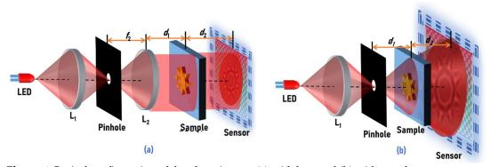
Figure. 1 Optical configuration of the phase imager (a) with lens and (b) without a lens.
