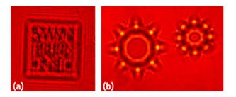
**Figure. 4** Intensity patterns recorded by the image sensor for (a) Swinburne logo with a lensless system and (b) stars with lens based system.
