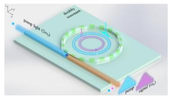
Fig. 1. Schematic of the quadratic soliton mode-locked DOPO. With the proper pump and cavity parameters, ultrashort pulses and broadband combs can be generated in cw-pumped doubly resonant cavities with quadratic nonlinearities.
