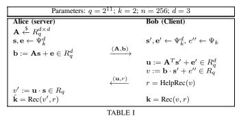
Key generation algorithm based on module-LWE
