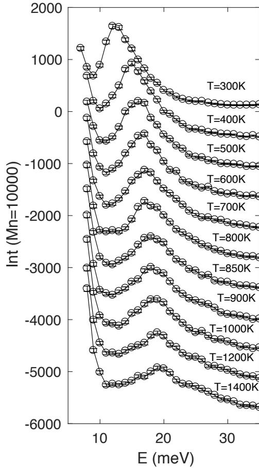
FIG. S5. Energy scans between 5 to 35 meV at  $Q = (2, 0, 0)$  from  $T = 300$  K to 1400 K for  $S_2$ . Curves are shifted for clarity. As temperature increases, the energy of the TO-mode shifts to higher energy. Energy scans have been fitted a damped harmonic oscillator convoluted with the spectrometer resolution. The temperature dependence of the energy peak position deduced from the fits is reported on Fig. 6 in the main text.
