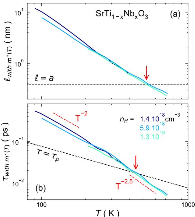
FIG. 7. Temperature dependence of the mean free path **a)** and of the scattering time **b)** for the three most dilute samples deduced from the resistivity data and the temperature-dependent effective mass obtained from the Seebeck data. With such a temperature dependent mass, the mean-free-path remains longer than the lattice parameter for  $T < 520$  K and the scattering time is longer than the planckian time for  $T < 450$  K. Both limits are violated at higher temperatures.
