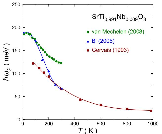
FIG. S2. Temperature dependency of the plasma frequency  $\omega_p$  extracted from a fit of the reflectivity spectrum by Gervais *et al.* [95] and Bi *et al.* [103] or by a fit of the Drude peak by van Mechelen *et al.* [104]. All three measurements are carried at the same Nb doping  $x = 0.009$  ( $n \sim 1.5 \cdot 10^{20} \text{ cm}^{-3}$ ).
