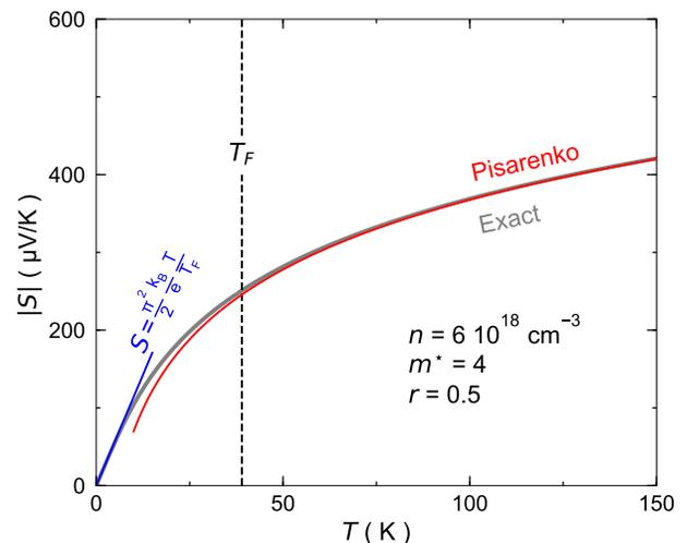
FIG. S3. Seebeck coefficient seen via different formulae: the low temperature approximation (in blue), the Pisarenko high temperature approximation (in red) computed from equation S9 and the exact derivation (in grey). The Pisarenko formula becomes valid with negligible error at the Fermi temperature  $T_F$ . Computation were done assuming a metal with  $n_H = 6 \times 10^{18} \text{ cm}^{-3}$ ,  $m^* = 4 m_e$  and a scattering parameter  $r = 0.5$  as stated on the figure.
