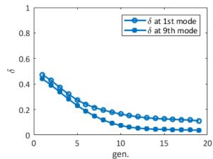
Fig. 8 Symmetric tree – Womersley's solution validity check as function of generation number for two different harmonic modes.
