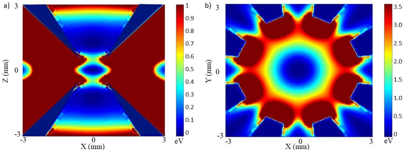
FIG. 2. Simulated RF pseudopotential of the trap with 800 V of RF at 12.4 MHz. a) XZ plane b) XY plane. The pseudopotential is symmetric about the Z axis and under  $45^\circ$  rotations in the XY plane. For these RF voltages and no DC confinement, we obtain  $\alpha=2.3$ . We note that a DC potential is necessary to increase the aspect ratio.
