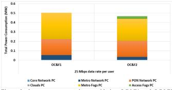
Figure 9: the power consumption considering OC&F1 and OC&F2 placement approaches. OC&F1 represents the optimal placement considering clouds and metro fogs only and OC&F2 represents the optimal placement considering clouds, metro and access fogs.
