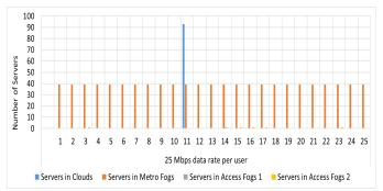
Figure 16: Number of servers required to host VMs of 40% minimum CPU workload under the OC&F approach with 25 Mbps data rate per user.
