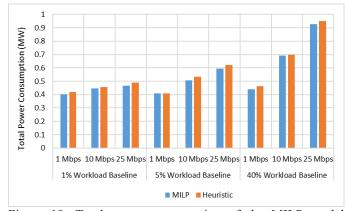
Figure 18: Total power consumption of the MILP model compared with EEVM-CF heuristics considering VMs with 1%, 5% and 40% CPU workload baseline.
