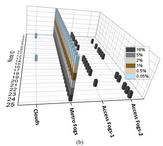
Figure 13: the optimal placement of different VMs popularity groups of 5% minimum CPU workload under the OC&F approach with 25 Mbps data rate per user.
