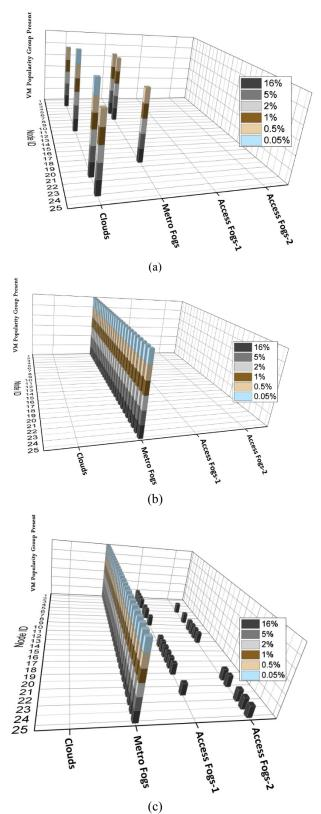
Figure 8: Optimal placement of different VMs popularity groups of 1% workload baseline under the OC&F approach with (a) 1 Mbps data rate per user, (b) 10 Mbps data rate per user and (c) 25 Mbps data rate per user.
