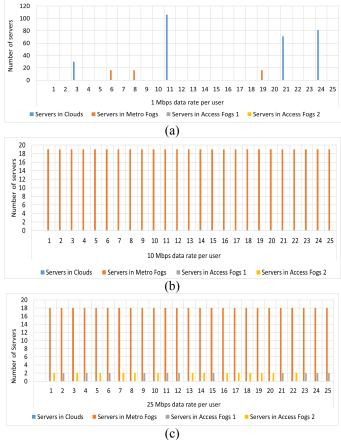
Figure 11: Number of servers in OC&F approach required to host VMs of 1% workload baseline with (a) 1 Mbps data rate per user (b) 10 Mbps data rate per user (c) 25 Mbps data rate per user.
