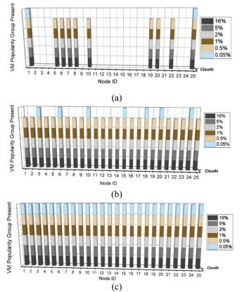
Figure 7: Optimal placement of different VMs popularity groups of 1% workload baseline under the OC approach with (a) 1 Mbps data rate per user, (b) 10 Mbps data rate per user and (c) 25 Mbps data rate per user.
