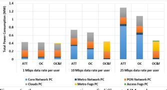
Figure 6: the power consumption of different VMs placement approaches considering VMs of 1% minimum CPU workload.
