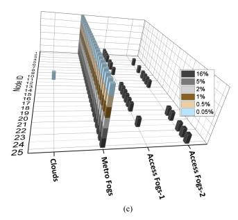
Figure 15: Optimal placement of different VMs popularity groups of 40% workload baseline under the OC&F approach with (a) 1 Mbps data rate per user, (b) 10 Mbps data rate per user and (c) 25 Mbps data rate per user.
