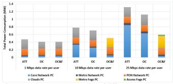
Figure 12: The power consumption of different VMs placement approaches considering VMs of 5% workload baseline.
