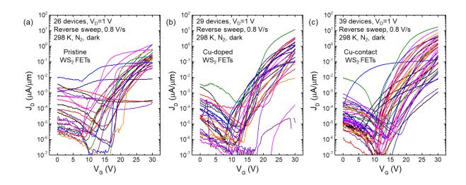
**Fig. S2** The transfer characteristics for (a) 26 pristine WS<sub>2</sub> FETs, (b) 29 Cu-doped WS<sub>2</sub> FETs, and (c) 39 Cu-contact WS<sub>2</sub> FETs.
