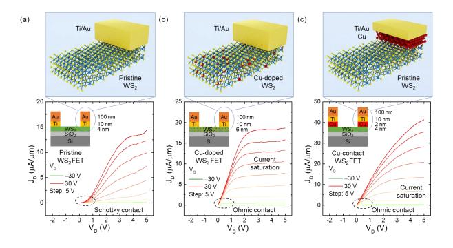
Fig. 2 Comparison of output characteristics of WS<sub>2</sub> FETs. (a, b, c) The output characteristics of pristine, Cu-doped, and Cu-contact WS<sub>2</sub> FETs at various  $V_G$  (from –30 to 30 V with a step of 5 V) at room temperature, respectively. Inset: Schematic illustration of the device structures and the corresponding metal-semiconductor interfaces.
