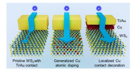
Fig. 1 Schematic illustration of generalized Cu atomic doping and localized Cu contact decoration on  $WS_2$  in a comparison with pristine  $WS_2$  with Ti/Au contact. The blue arrow indicates the electron injection through the metal-semiconductor interface.
