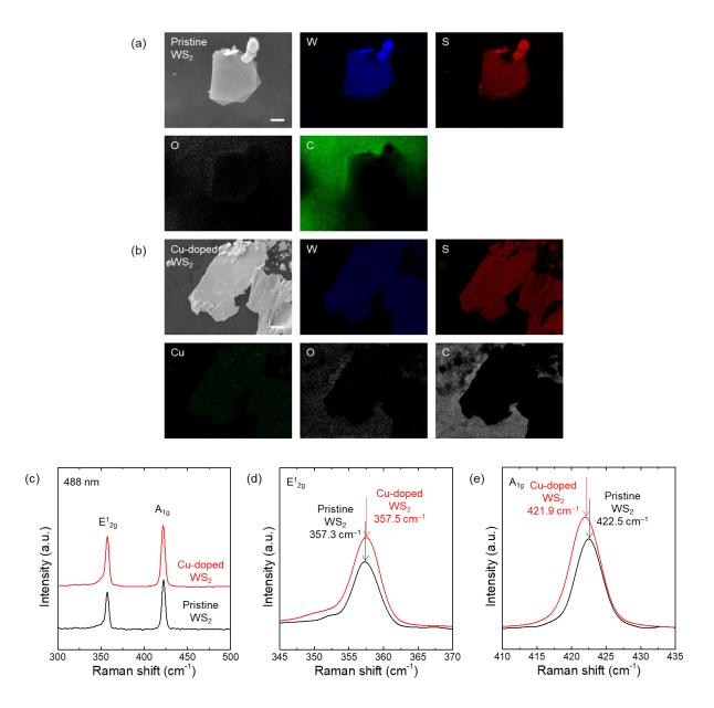
Fig. S3 (a, b) SEM and EDX elemental mapping of a synthesized pristine  $WS_2$  flake and a Cudoped  $WS_2$  flake transferred on the carbon tape surface. Scale bar: 2  $\mu$ m. (c-e) Raman spectroscopy of the pristine and Cu-doped  $WS_2$ .
