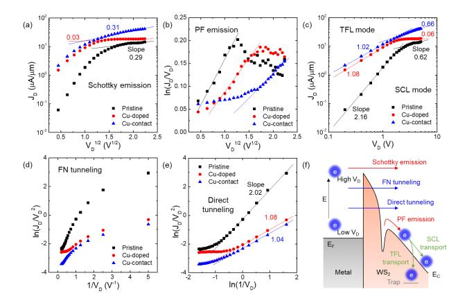
**Fig. S1** *IV* characteristics of WS<sub>2</sub> FETs at on state ( $V_G = 30$  V) based on the output curves. Various models, including (a) Schottky emission model, (b) PF emission model, (c) TFL/SCL model, (d) FN tunneling model, and (e) direct tunneling model were used for comparative investigation. (f) Energy band diagram at the metal-semiconductor interface illustrates the mechanisms of the carrier injection and transport.
